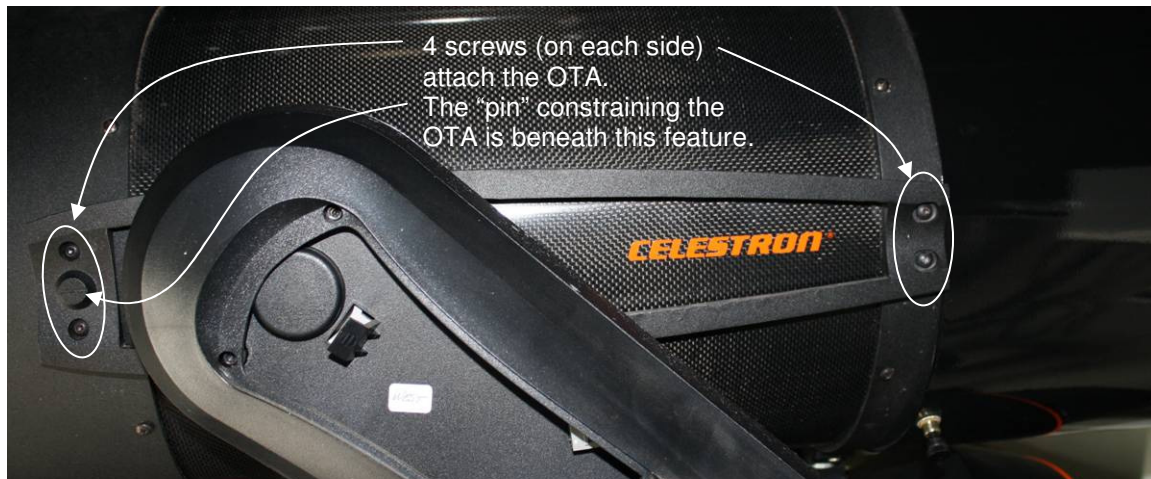
Figure 5: Bracket holds the Optical Tube Assembly
