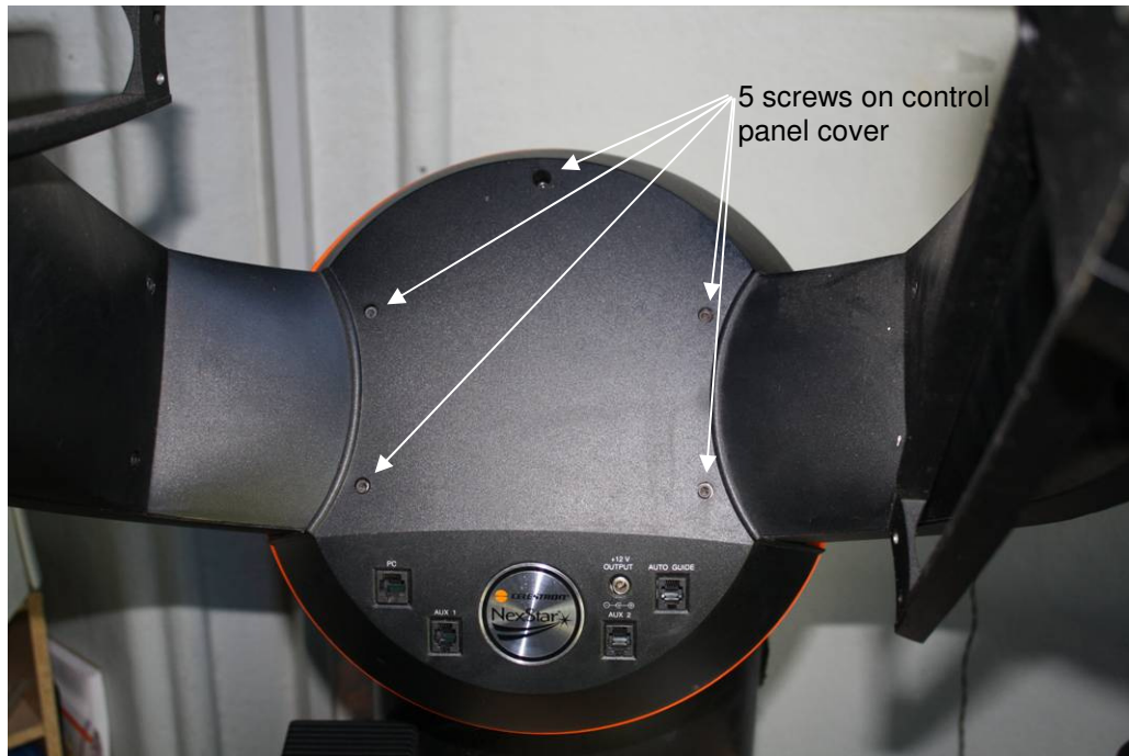
Figure 8: Control panel cover
